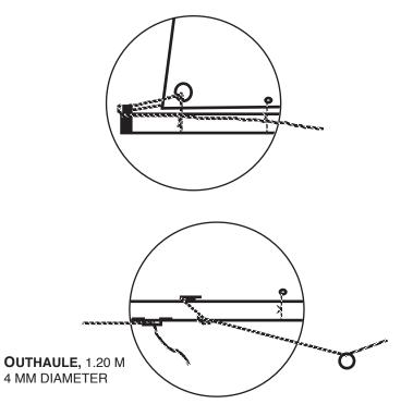
**BRIDLE**, 1.42 M, 3 MM DIAMETER WITH STAINLESS STEEL RING FOR MAINSHEET. ATTACH THE BRIDLE TO THE BOOM WITH A BOWLINE KNOT.
